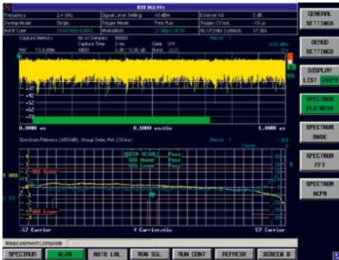
Spectrum flatness and group delay of the 104 occupied carriers of a 40 MHz wide IEEE802.11n signal (Greenfield mode).
